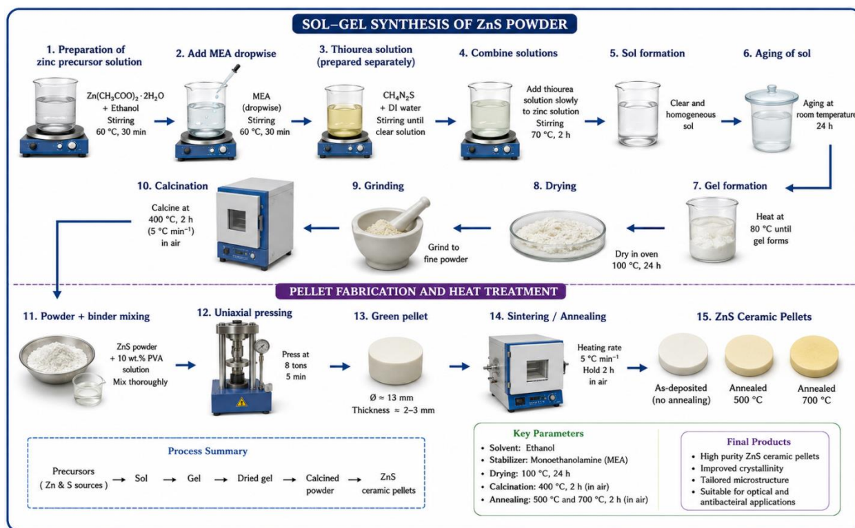
Fig. 1. Schematic illustration of the preparation procedure of ZnS ceramic materials via the sol-gel method.
