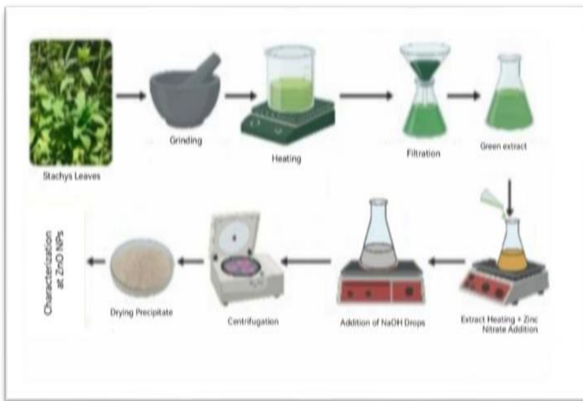
Figure 1. Schematic representation of the green synthesis mechanism of ZnO nanoparticles using Stachys leaf extract.
